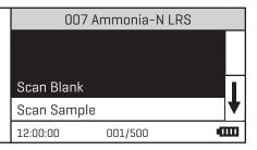
6. Insert the reacted sample into the chamber. Close the lid. Press enter to scan the sample. The screen will display **Scan Sample Sample Done** for about 1 second. The result will appear on the screen.
