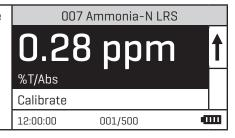
8. Press ENTER to select **Calibrate**. A reverse font (light background with dark characters) will appear to indicate that the reading can be adjusted.
