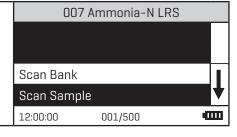
5. Insert the blank into the chamber. Close the lid.Press to scan the blank. The screen wil display **Scan Blank Blank Done** for about 1 second and then return to the test menu.
