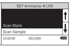
6. Insert the reacted standard solution into the chamber. Close the lid. Press ENTER to scan the sample. The screen will display Scan Sample Sample Done for about 1 second. The result will appear on the screen.
