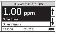
To repeat the test, press ENTER to scan the sample again. The last blank scanned is used by the colorimeter for repeated scans.
