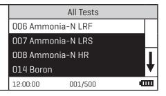
3. Press or to scroll to the desired test.
