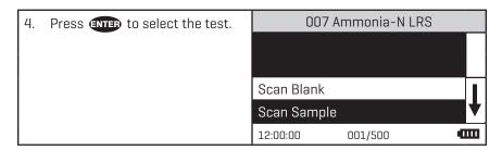
5. Follow the test procedure in the manual to test the prepared standard. Insert the blank into the chamber. Close the lid. Press enter to scan the blank. The screen will display Scan Blank Blank Done for about 1 second and then return to the Test Menu.
